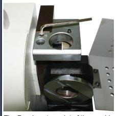
The Dead centre point of the machine can be set by using the allen screws under the grinding wheel cover. (as shown)
